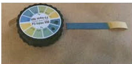
Fig. 6 The concentration (2%) of P3-topax-990 was checked with indicator paper specially provided by Ecolab (at the starting point, At half way and at the end of the test ).
